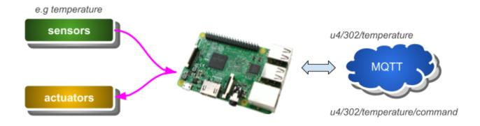
In the upper example, the device is a Raspberry Pi that could be connected to either a wired / wireless network. Each kind of sensor / actuator maps to a topic class. However, to be able to publish / subscribe to the MQTT broker, the device's client needs credentials. To obtain these credentials, you first need to:
