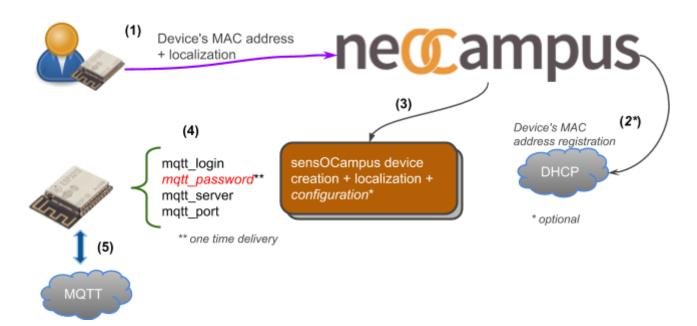
sensOCampus is the main end-devices management application developed for neOCampus. It takes care of managing the device's own specific setup (MAC, configuration, status, topics etc).
