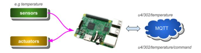
In the upper example, the device is a Raspberry Pi that could be connected to either a wired / wireless network. Each kind of sensor / actuators map to a topic class. However, to be able to publish / subscribe to the MQTT broker, the device's client needs credentials. To obtain these credentials, you first need to:
