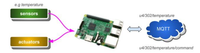
In the upper example, the device is a Raspberry Pi that could be connected to either a wired / wireless network. Each kind of sensor / actuators map to a topic class. However, to be able to publish / subscribe to the MQTT broker, the device's client needs credentials. To obtain these credentials, you first need to:
