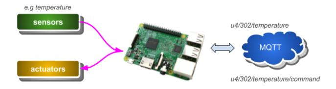
In upper example, device is a Raspberry Pi that could be connected to either a wired / wireless network. Each kind of sensors / actuators map to a topic class. However, to be able to publish / subscribe to the MQTT broker, device's client needs credentials. To obtain these credentials, you first need to:
