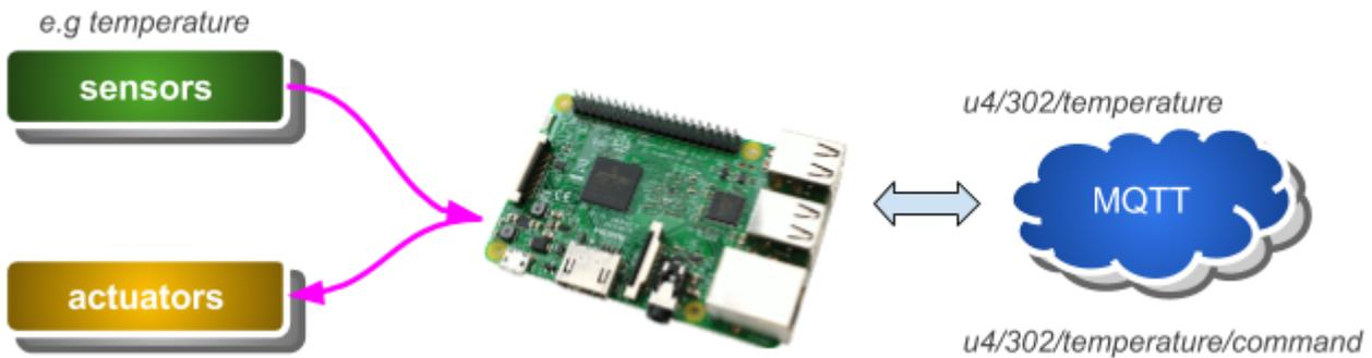
In upper example, device is a Raspberry Pi that could be connected to either a wired / wireless network. Each kind of sensors / actuators map to a topic class. However, to be able to publish / subscribe to the MQTT broker, device's client needs credentials. To obtain these credentials, you first need to:
