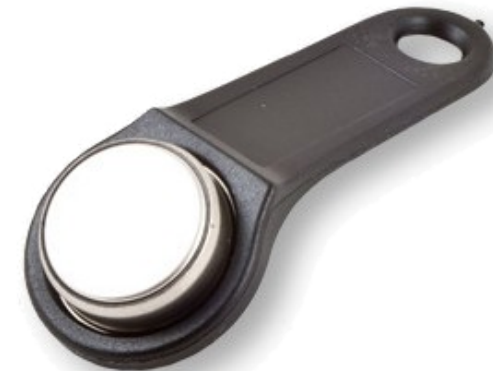
iButton is 1-wire powered.
