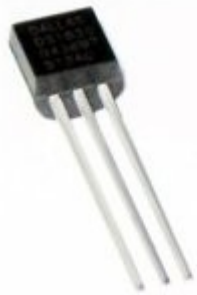
1-wire temperature sensor Dallas 1820B.
